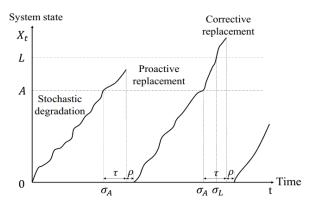
Figure 1 Sketch of degradation model and maintenance policy with stochastic process.
