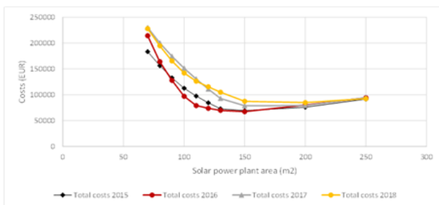
Figure 3: Cost optimisation in consecutive years for a specific location of family house with solar power plant and battery.
